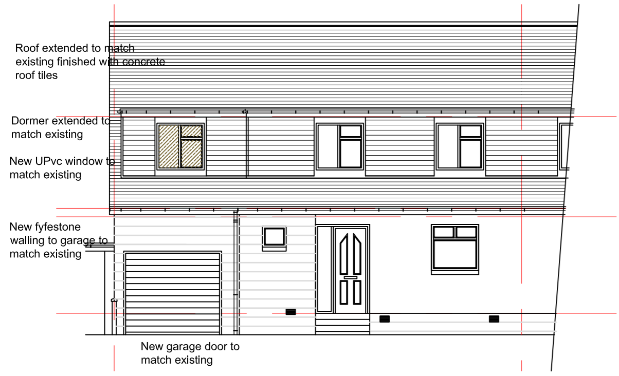
Front Elevation as Proposed Scale 1/100
